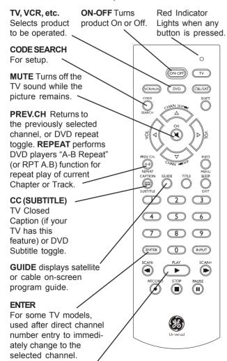
RECORD, PLAY, STOP, REW, FF, PAUSE VCR control buttons operate your VCR even when the remote is set to operate the TV. Also operates DVD Scan -/+. Note the VCR keys also control DVD when in DVD Mode.
